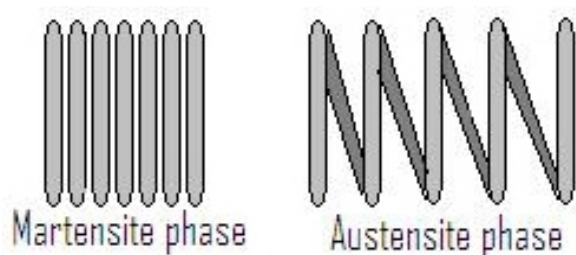
Fig. 1: Different Phases of SMA
